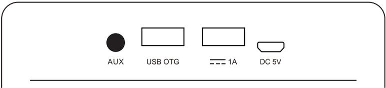
Use the included 3.5mm audio cable to connect an external device to the AUX input jack (10). Press the “MODE” button (1) until the LED indicator (7) turns red confirming AUX has been selected as sound source.
