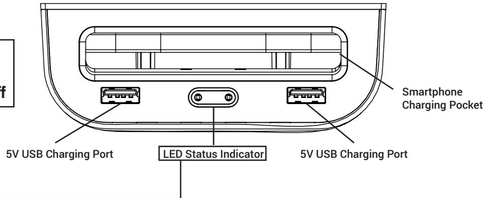
*Note: Place smartphone in pocket with screen facing away from LED Status Indicator to charge.*
