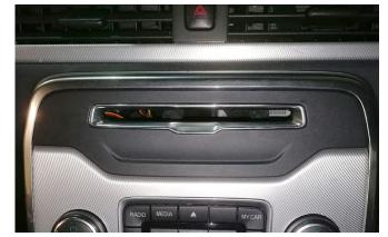
Disengage the CD slot plastic housing by bending in the clips on the inside of the slot with a panel removal tool.
