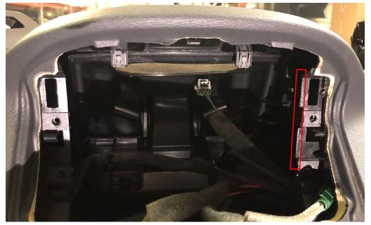
The highlighted section of dashboard frame will need to be filed down (roughly 2mm) in order for a new double DIN unit to sit in place correctly.
