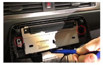
Once the main panel is removed, undo the 2x bolts on either side of the main head unit. When done, remove completely whilst disconnecting all of the wiring.
