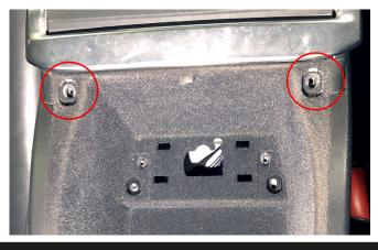
Open the centre console armrest and use the panel removal tool to help remove the rubber grommets that cover the following screws. Once uncovered, remove the 2x Torx screws.
