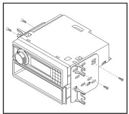
With the pocket roughly attached, take the new radio and place it into the remaining area in between the brackets and screw it into place using the 2x left over screws. Ensure that the metal sleeve has been removed from around the radio before screwing into place.
