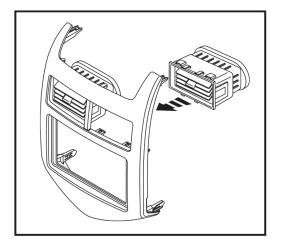
Take the original fascia in hand and use a panel removal tool to unclip the 2x air vents. Then proceed to implant these air vents into the appropriate ports on the CT23CV07 fascia.
