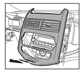
Begin by using a panel removal tool to unclip the main fascia panel. Once free, remove fully from the dashboard.
