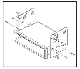
When installing a single DIN radio, take the brackets and 2x of the screws and attach them to either side of the pocket found within the kit. The location (top or bottom) is dependent on the consumer.
