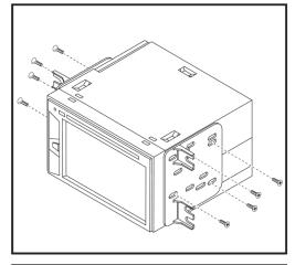
When installing a double DIN radio, take the brackets and all 4x screws from within the kit and attach them to the relevant sides of the radio.
