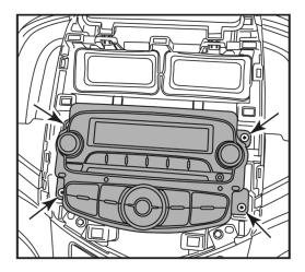
With the main fascia out of the way, proceed to undo the 4x screws that secure the main head unit in place. Once free, pull it out of the dash and disconnect all of the wiring.
