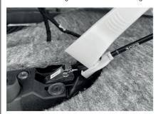
Disconnect electrical connections for the window control panel
