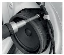
Use the pry tool to release the speaker from the door.
