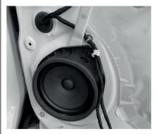
Release the clips that hold the speaker cable to the basket and release the speaker connector.
