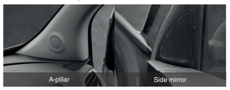
Start by removing the tweeter covers. Use plastic pry tools and be careful, there can be air-bags behind the A-pillar. The first clip can be hard to remove. Take it easy and use minimal force. The instructions below shows how to remove the A-pillar tweeter.
