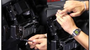
Unscrew the eight screws holding the head unit and top display in place.
