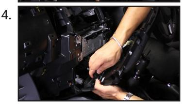
Once the fascia panel is free, disconnect all wiring to the panel and remove the panel.
