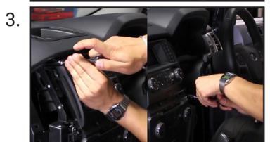
With the panels removed, use a screwdriver to remove the five screws holding the fascia panel in place.
