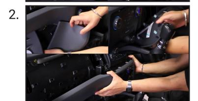
Next, remove the panels underneath the A/C controls by hand, followed by the panel situated between the head unit and A/C controls.
