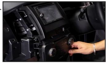
Now reconnect all connections to the fascia panel and air conditioning assembly and clip into place around the head unit.
