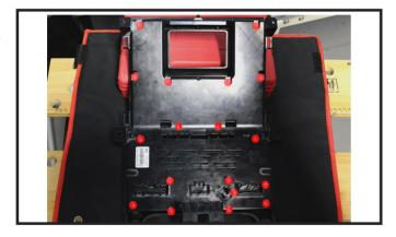
Take the OEM fascia panel and remove all eighteen screws located on the back (see circled images opposite).
